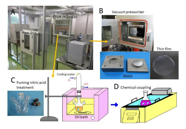
**Fig. 3.** Clean room facility for manufacturing of artificial retina OUReP. Ceiling and walls of clean room are made by transparent acrylic boards (**A**). Polyethylene thin film is produced by mold in vacuum pressurizer (**B**), treated with fuming nitric acid to induce surface carboxyl group (**C**), and chemically coupled with ethylene diamine and then with photoelectric dye (**D**).
