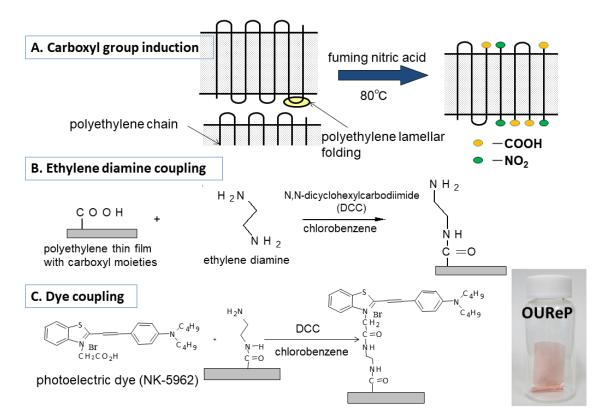
**Fig. 1.** Chemical process to produce photoelectric dye-coupled polyethylene thin film as artificial retina OUReP. Carboxyl group (COOH) is induced on polyethylene thin film surface by fuming nitric acid treatment ( $\mathbf{A}$ ), ethylene diamine is coupled to carboxyl group on the film surface ( $\mathbf{B}$ ), and then photoelectric dye is bonded ( $\mathbf{C}$ ).
