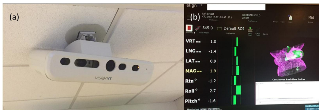
Figure 7. Optical surface tracking system (a) optical camera mounted on the ceiling of the treatment room (see Figures 4(a) and 5) (b) User interface showing patient setup instructions
